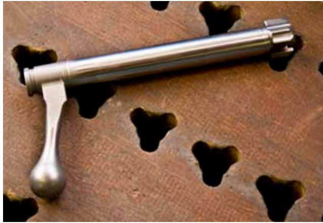
Cast as a single piece, this L-shaped component will become a bolt for a Sako 85. Sako still uses many of the same machines, wooden organizers and tools that originally built the company's reputation.
