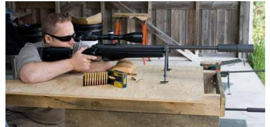
A quiet kind of precision: For discreet target practice, the use of suppressors is encouraged throughout Europe. Here, the author shoots a suppressed .308 Sako TRG-22 from its bipod. He averaged 0.98-inch five-shot groups on five targets at 100 meters.
