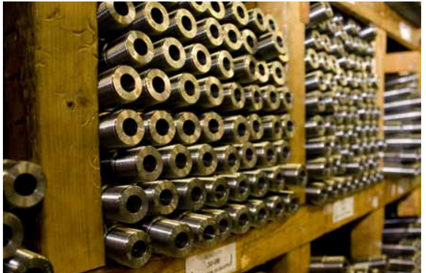
Clearly organized in a wall of wooden shelving, Sako barrels are hammer forged, polished and finished at the factory. Calibers currently range from .204 Ruger to .375 H&H.
