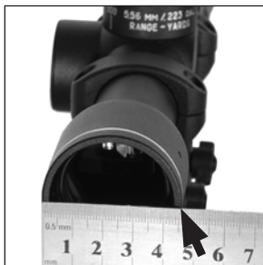
FIGURE C-1. OBJECTIVE TUBE DIAMETER MEASURING
