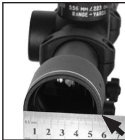
FIGURE B-1. OBJECTIVE TUBE DIAMETER MEASURING
