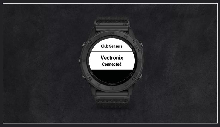
When the connection between a Garmin tactix<sup>®</sup> Delta Solar and your TERRAPIN X is successful, the Bluetooth symbol is displayed continuously in your TERRAPIN X and in the display of the watch the message «Vectronix Connected» appears.
