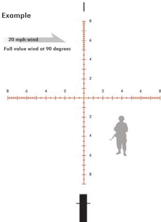
Using 3 mrad drop line at 500 yards, 4.0 mrad correction for 20 mph wind.
