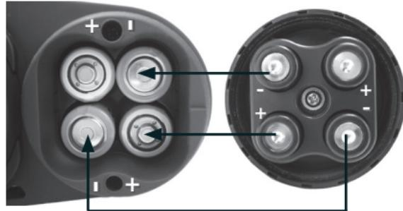
Observe battery polarity marks inside battery compartment when inserting batteries, and ensure polarity marks on cap match polarity in battery compartment when replacing cap (+ to + and - to -).
