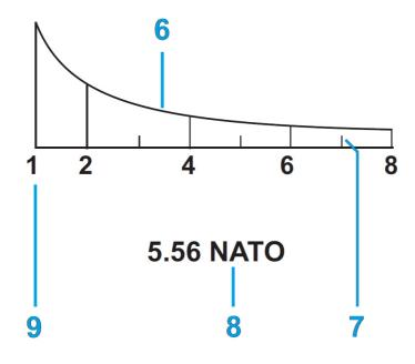
**6** The range mark is configured for a target height of 1 m. **9** The numerical values within the curve indicate the distance to the target in m.
