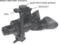
FIGURE 2-14. ADAPTER TO MIL-SPEC HEAD/HELMET
