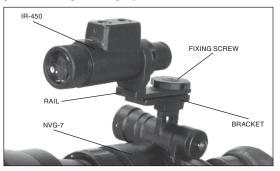
FIGURE 2-13, IR450 INSTALLATION
