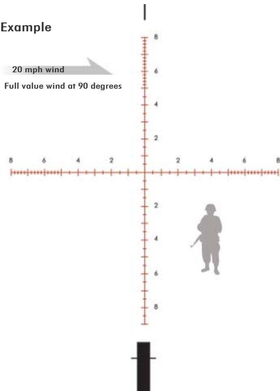
Using 3 mrad drop line at 500 yards, 4.0 mrad correction for 20 mph wind.
