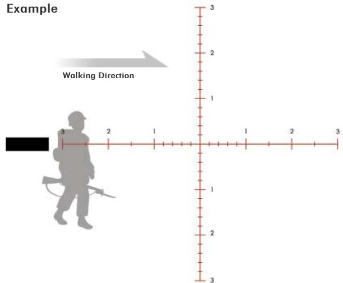
2.74 mrad correction for a man walking at 3 mph at 800 yards. No wind. Total bullet time of flight from trigger pull 1.5 seconds during which man travels 6.6 feet. Elevation already dialed into turret.
