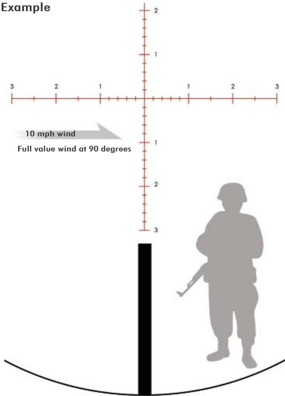
Using 3 mrad drop line at 500 yards, 2 mrad correction for 10 mph wind.
