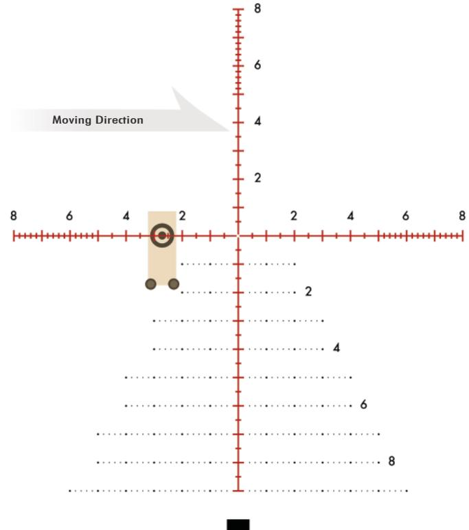
*2.74 mrad reticle correction for a target moving at 3 mph at a distance of 800 yards. No wind. Total bullet time of flight from moment of trigger pull is 1.5 seconds during which a target travels 6.6 feet. Elevation already dialed into turret.*
