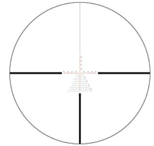
lead corrections. Ultra precision laser etching on the glass reticle ensures that mrad specifications can be kept to the tightest tolerances possible. The fine center crosshair subtensions on the EBR-2 mrad reticle were carefully chosen to provide the optimum balance between precision aiming and low light visibility.
